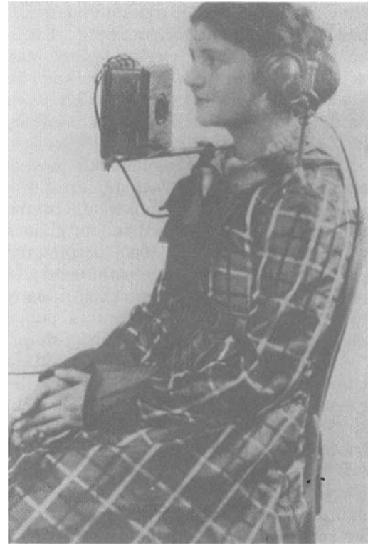
Figure 3.14 The early headsets worn by telephone operators could weigh more than six pounds.
