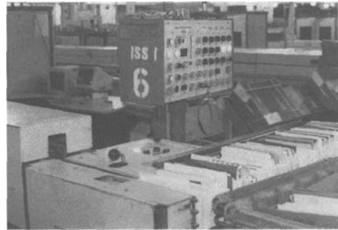
Figure 5.3 A modern Post Office optical character reader automatically identifies the numbers in a ZIP code.
